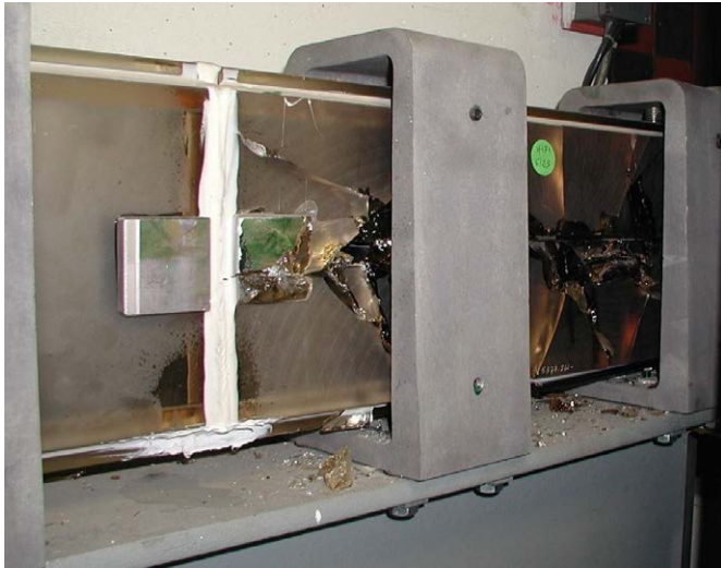
(a) H17 guide after implosion
