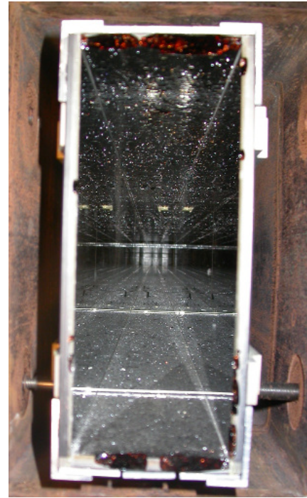
(b) H113 guide, peeling of the mirrors
