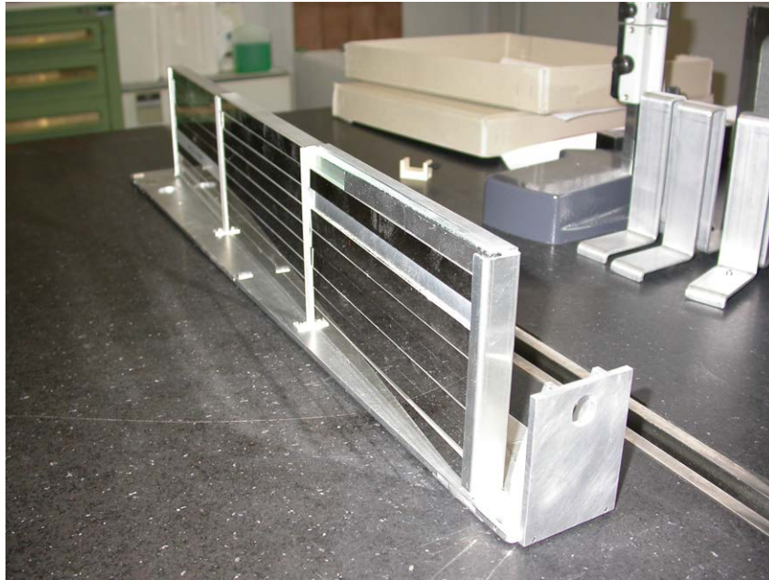
Figure 2.9: Sample holder used for irradiation at the H112 and H21 guides. View from the back. The insertion in a neutron guide is done by pushing on the vertical aluminium plate on the forefront of the picture
